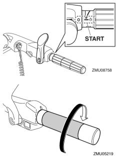
(2) After the engine is at idle speed in gear move the remote control lever / gear shift lever firmly and crisply into the neutral position.
