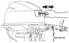
(5) After the engine starts, slowly return the manual starter handle to its original position before releasing it.
