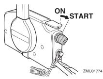
(5) Immediately after the engine starts, release the main switch and allow it to return to "ON" (on). NOTICE: Never turn the main switch to "START" (start) while the engine is running. Do not keep the starter motor turning for more than 5 seconds. If the starter motor is turned continuously for more than 5 seconds, the battery will be quickly discharged, thus making it impossible to start the engine. The starter can also be damaged. If the
