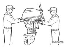
(4) Mount the outboard motor on the center line (keel line) of the boat, and ensure that the boat itself is well balanced. Otherwise the boat will be hard to steer. For boats without a keel or which are asymmetrical, consult your dealer.
