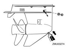
(6) Put a new gasket on the oil level plug. When the oil begins to flow out of the oil level plug hole, insert and tighten the oil level plug.
