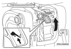
(3) Slightly tilt the outboard motor up. The tilt support bar will lock automatically, supporting the outboard motor in a partially raised position. This outboard motor has 2 positions for shallow water cruising.
