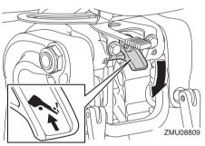
(2) Slightly tilt the engine up until the tilt support bar is automatically released.
