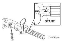
(4) Pull the manual starter handle slowly until you feel resistance. Then give a strong pull straight out to crank and start the engine. Repeat if necessary.
