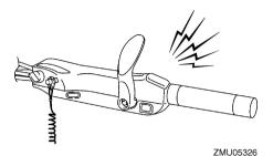
If the alert system has activated, stop the engine as soon as it is safe to do so. Check the oil level and add oil as needed. If the oil level is correct, consult your Yamaha dealer.
