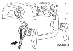
(3) Secure the clamp bracket to the transom using the bolts provided with the outboard (if packed). For details, consult your Yamaha dealer. WARNING! Avoid using bolts, nuts or washers other
