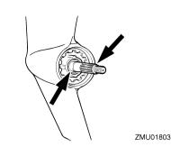
Check the propeller shaft oil seal for damage.
