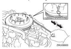
(6) Pull the rope slowly until resistance is felt. Give a strong pull straight out to crank and start the engine. If the engine does not start on the first try, repeat the procedure.
