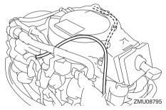
(4) Be sure that the gear shift is in neutral and that the clip is attached to the engine shut-off switch.
