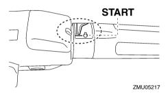
(4) Turn the main switch to "START" (start), and hold it for a maximum of 5 seconds.
