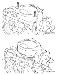
(3) Pass the start-in-gear protection cable under the blow by hose and remove the spring from it.
