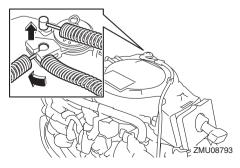
(2) Remove the manual starter after removing the bolt(s).
