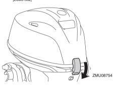
After installing, check the fitting of the top cowling by pushing it with both hands. If the top cowling is loose, have it repaired by your Yamaha dealer.
