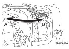
If the resistance does not increase even when the lever is turned to the starboard side "A", make sure that the nut is tightened to the specified torque.
