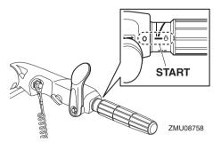
(4) Push the starter button to start the engine.
