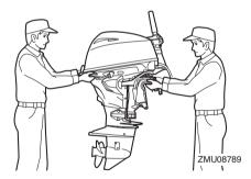
(7) When transporting or storing the outboard motor while removed from a boat, keep the outboard motor in the attitude shown or use an outboard motor stand.
